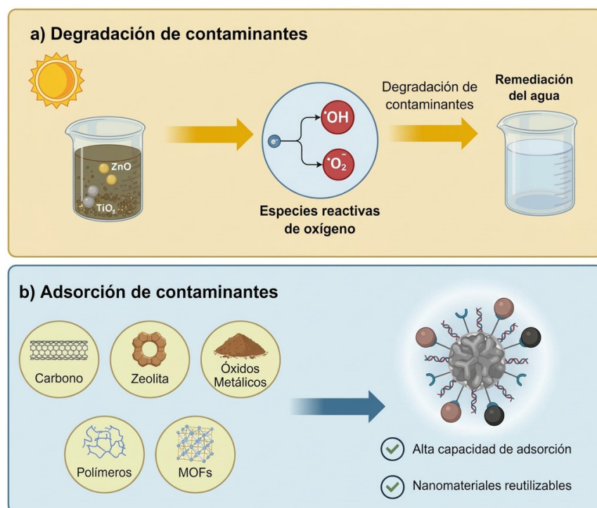
Figura 5. Aplicaciones de la nanotecnología verde en la remediación ambiental: a) degradación fotocatalítica de contaminantes mediante especies reactivas de oxígeno (ROS); b) adsorción de contaminantes mediante nanoadsorbentes de carbono, zeolitas, óxidos metálicos, polímeros y MOFs. Basado en Zakir et al., J. Water Process Eng. 2025; Hussein et al., RSC Adv. 2025; Asghar et al., J. Nanobiotechnol. 2024; Lu, Catalysts 2025. Basado en Zakir, O.; Ait-Karra, A.; Khardazi, S.; Idouhli, R.; Khadiri, M. E.; Dikici, B.; Aboulaich, A.; Outzourhit, A.; Abouelfida, A. Recent Progress in Nanomaterials for Water Treatment: A Comprehensive Review of Adsorption, Photocatalytic, and Antibacterial Applications. Journal of Water Process Engineering 2025, 72, 107566; Hussein, E. B.; Rasheed, F. A.; Mohammed, A. S.; Kayani, K. F. Emerging Nanotechnology Approaches for Sustainable Water Treatment and Heavy Metals Removal: A Comprehensive Review. RSC Adv. 2025, 15 (48), 41061–41107; Asghar, N.; Hussain, A.; Nguyen, D. A.; Ali, S.; Hussain, I.; Junejo, A.; Ali, A. Advancement in Nanomaterials for Environmental Pollutants Remediation: A Systematic Review on Bibliometrics Analysis, Material Types, Synthesis Pathways, and Related Mechanisms. J Nanobiotechnol 2024, 22 (1), 26; Lu, X. Photocatalytic Nanomaterials for Environmental Purification. Catalysts 2025, 16 (1), 13
